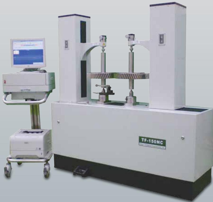
CNC Single flank gear rolling tester
